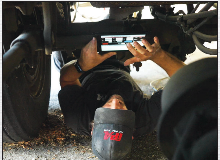
One-Man ABS Diagnostics with Tablet
